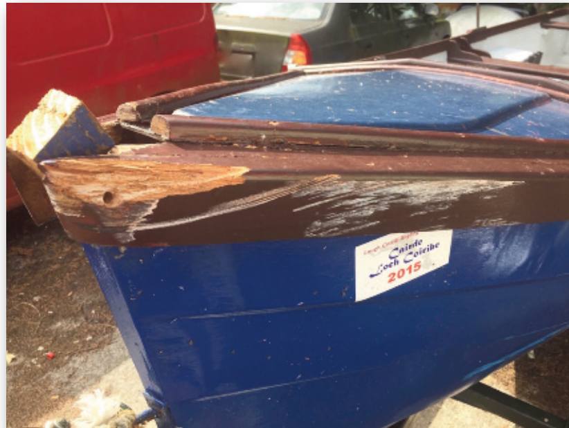
Photograph No. 4: Close-up view of damage to stem, port side gunwales and opening of join to breast hook/weather deck.
