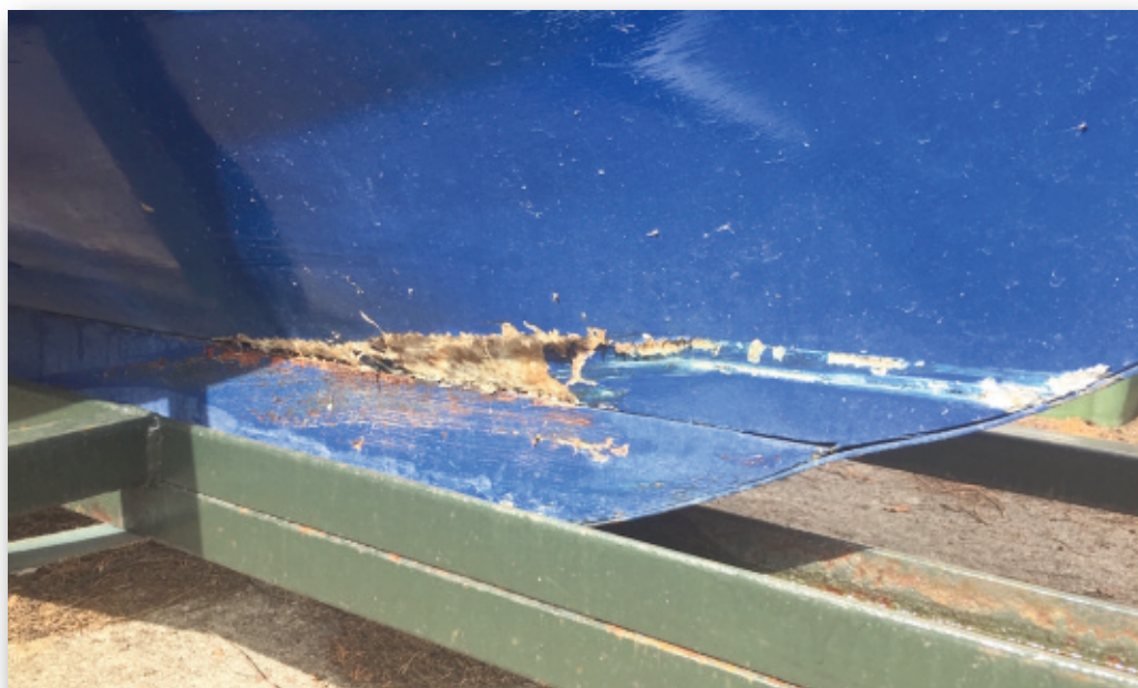
Photograph No.6: Damage to starboard side forward part of keel and garboard strake.
