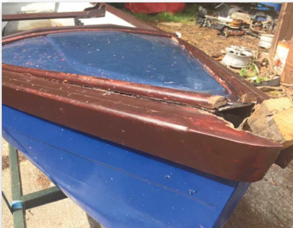
Photograph No. 5: Opening up of breast hook/weather deck on starboard side.
